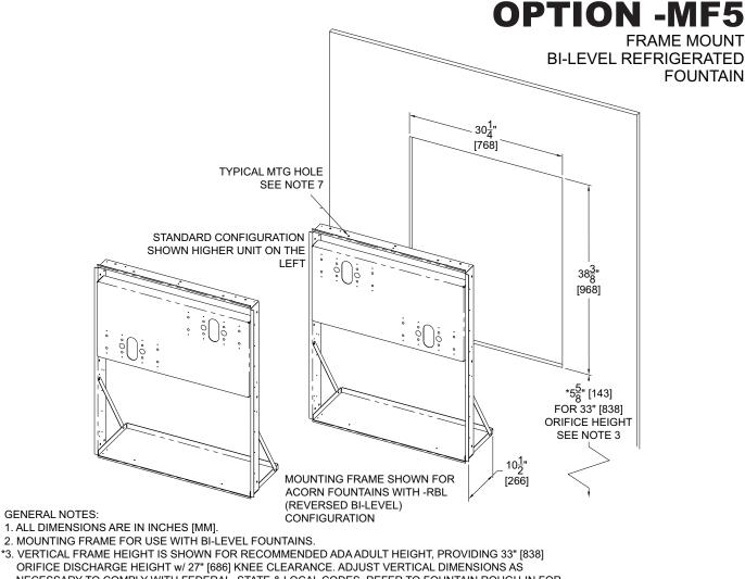
ORIFICE DISCHARGE HEIGHT w/ 27" [686] KNEE CLEARANCE. ADJUST VERTICAL DIMENSIONS AS NECESSARY TO COMPLY WITH FEDERAL, STATE & LOCAL CODES. REFER TO FOUNTAIN ROUGH-IN FOR MORE DETAILS ON FIXTURE.
