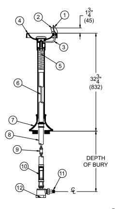
\* Valve specifications: Minimum/Maximum Pressure 30 to 100 psi.
