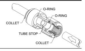
2. Pull on the fitted tubing to ensure it is secure. Tube should not come free from the fitting. Water test the connection assembly prior to leaving the site to ensure there are no leaks.
