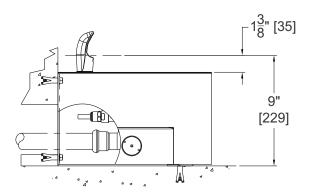
\* Valve specifications: Minimum/Maximum Pressure 30 to 100 psi.
