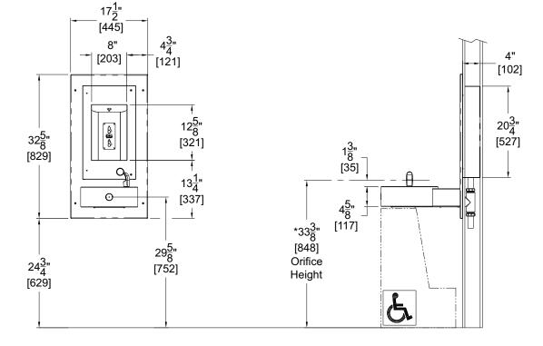
**NOTES:** Dimensions shown for Adult ADA compliant installation. For Child ADA compliant parallel approach installation, decrease height of installation by 3 inches. Provide clear floor space as required. Adjust vertical dimensions as required to comply with federal, state, and local codes.
